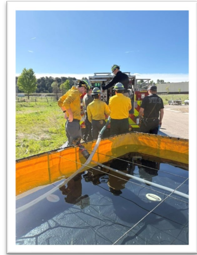
Photo of new members learning to draft a brush truck from a portable water tank.
